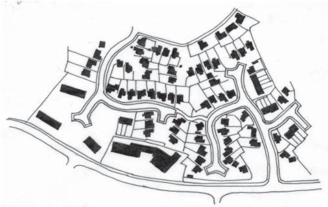
Fig. 7. Plan of cul-de-sac design that increases segregation and reduces interaction of communities and surroundings.
