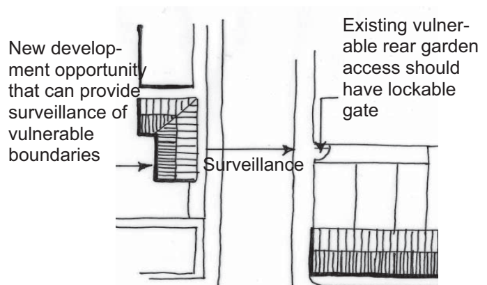
Fig. 26. Surveillance of vulnerable rear garden access.
