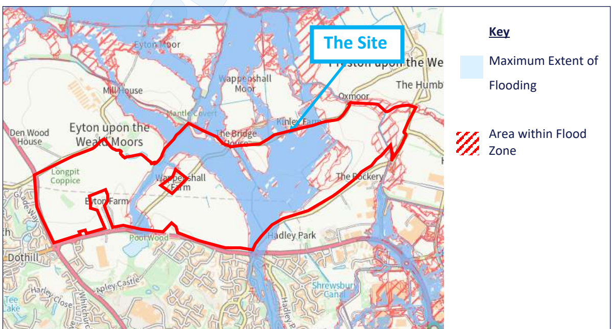
Figure 5-6: EA Long Term Flood Risk Maps – Flood risk from Reservoirs (Gov.Uk webSite)
